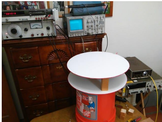
Figure 4. Picture of the two round coil forms employed in an experiment with induction.
