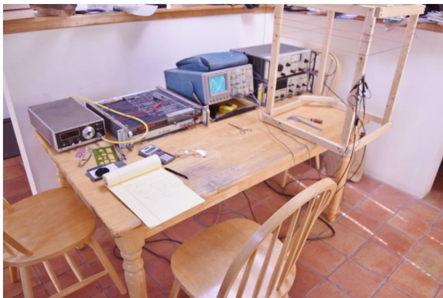
Figure 2. Picture of square coil form used for testing induction. Also pictured is the test equipment employed in the experiment.
