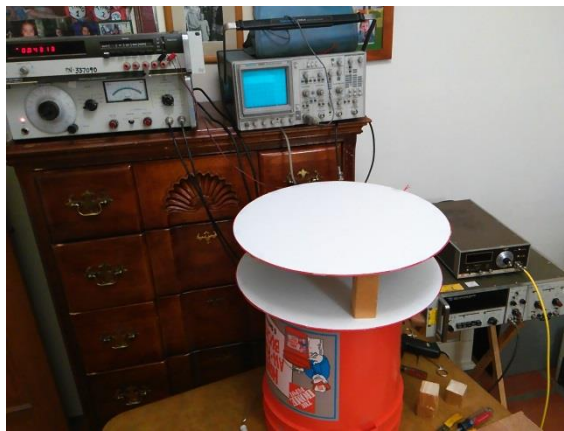
Figure 7. Picture of the two round coil forms employed in an experiment with induction.
